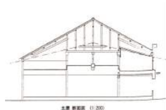
Fig.3.68 Structure with old and new ridgepoles, drawn in the survey from 2012. Source: Kurayoshi city.
