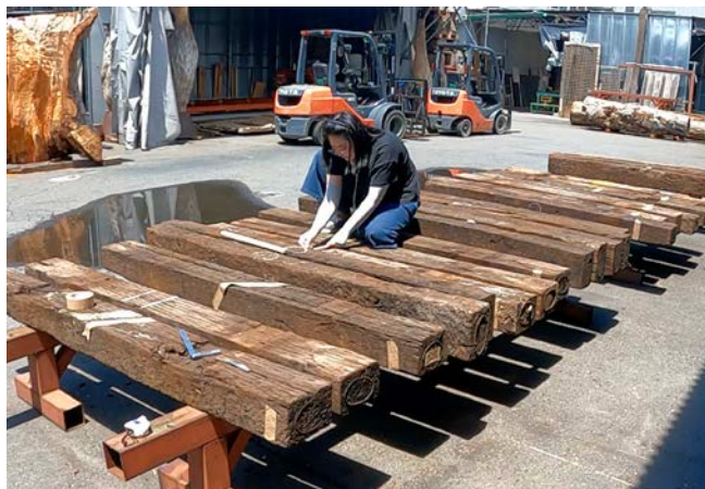
Assessing the Twist and Height of Sleepers
