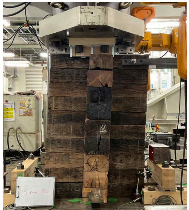
Vertical Load 100 kN, Inter-Story Drift Angle 1/15 rad, Negative Direction
